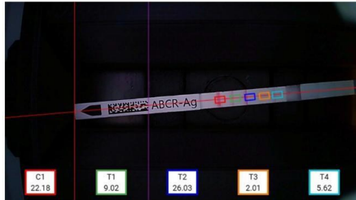
Figure 4. Test strip inserted in the maximum angle in the tray showing that the iaX adjusts the reading area accordingly and analyses the results correctly.
